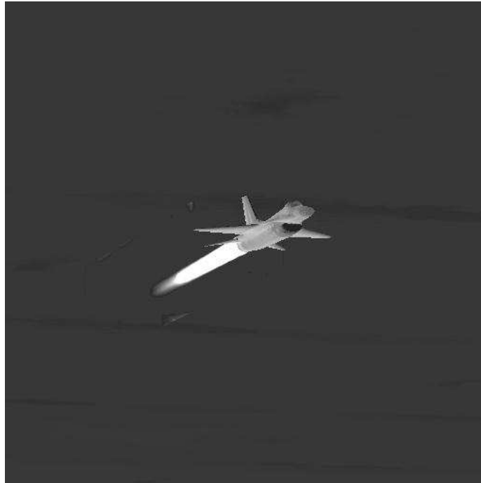
Figure 7. MWIR image computed using SE-RAY-IR and SE-SPECIAL-EFFECTS
