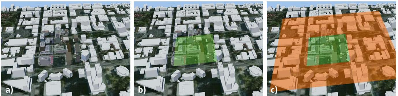
**Figure 4. The San Jose model contained most of the details around the receiver antenna (b), whilst in only height correction for the building far from the antenna (c).**
