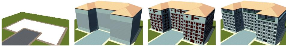
Figure 1 From left to right: Entry data (building footprint), first derivation step, setting up extrusions and final building.
