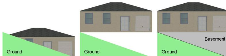
Figure 10: The three different kinds of groundwork templates. From left to right, zMin, zMax and Extruded
