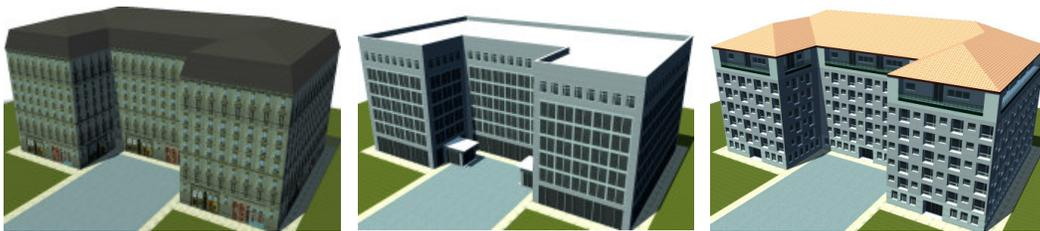
Figure 13: Three different buildings generated from the same building footprint. Left: a Hausman building with a mansard roof (94 faces). Middle: a glass building, with 2 external objects for the entry hall and a flat roof (350 faces). Right: a highly extruded building with a four-sloped roof (5600 faces).
