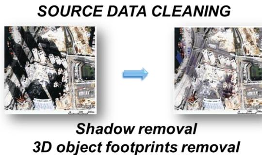
Figure 21. Example of ortho-image cleaning
