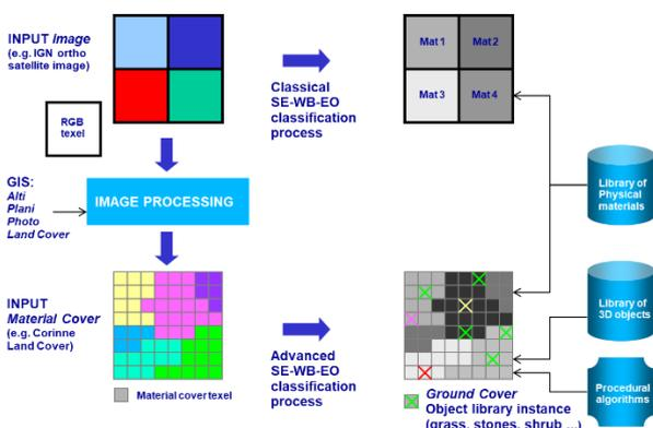
Figure 25. 3 ways to use texture in SE-WB: Classical classification, Material Cover & Ground Cover
