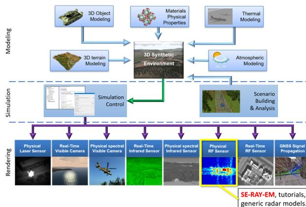
Figure 2: Global architecture of OKTAL-SE SE-Workbench
