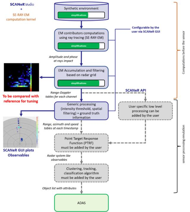
Figure 6: Optimized level - processing steps
