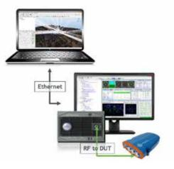
FIGURE 2 System diagram that shows propagation simulator controller (top), the GNSS simulator (bottom), and the device under test connected to the RF output of the simulator.
