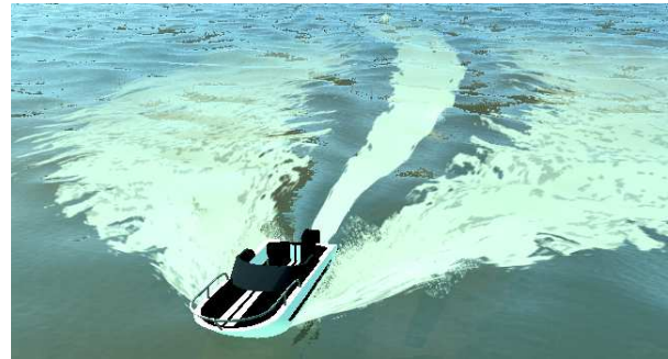
Figure 12: Example of wake simulation using SE-RAY
