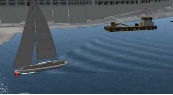
Figure 14: Example of wake simulation using SE-FAST
