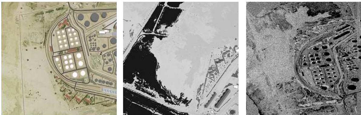
**Figure 1:** Illustration of the main principle of the SE-WORKBENCH: generation of multi-sensor images from the same 3D environment: Visible spectral domain (left), Infrared-EO domain (middle), radio-frequency SAR domain (right).
