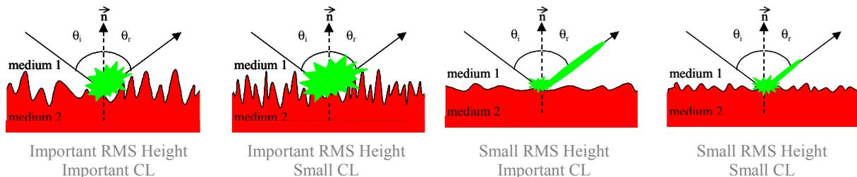
**Figure 4:** Illustration of the main principle and parameters of the He Torrance model.
