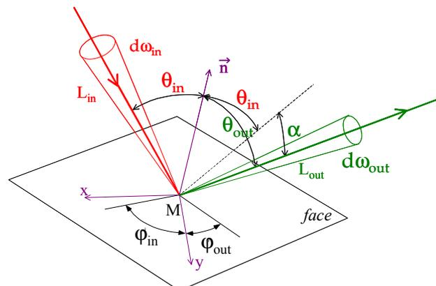
The BRDF (Bi-directional Reflectance Distribution Function) is the only serious data that can be used in physical simulation. It is defined aside. Integration is performed on the solid angle  $d\omega_i$  corresponding to the source visibility from the reflection point.
