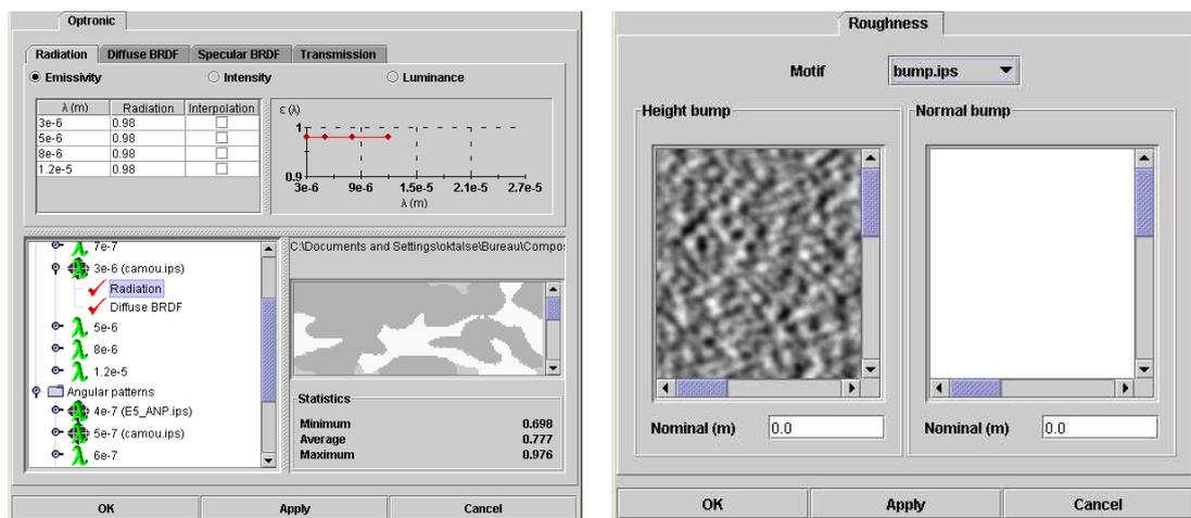
**Figure 2:** User interface of the SE-PHYSICAL-MODELER software: Schematic Infrared material physical properties edition (left), Surface state material properties edition (right).
