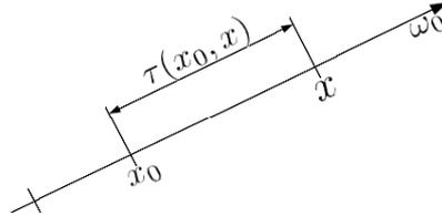
Figure 10: Geometry associated to the volume transfer equation
