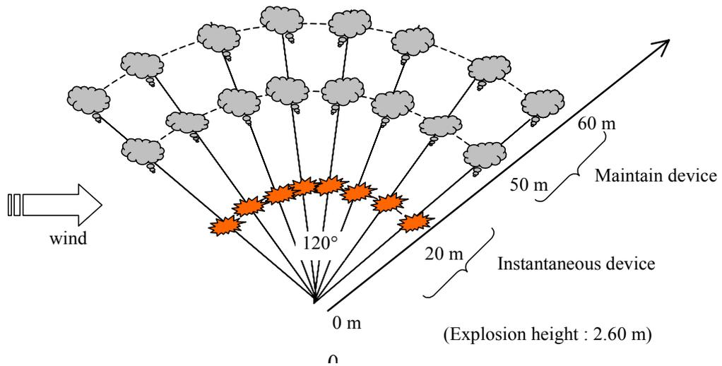
Figure 2: Example of positions of pyrotechnical devices
