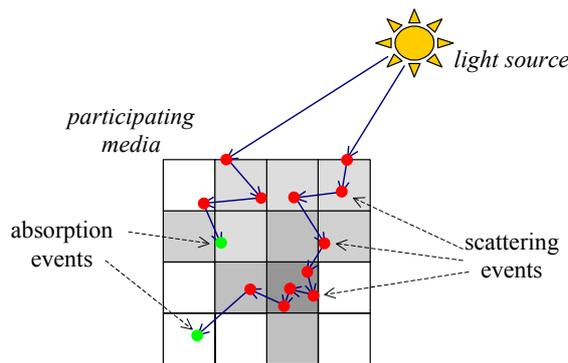
Figure 11: Photons propagation
