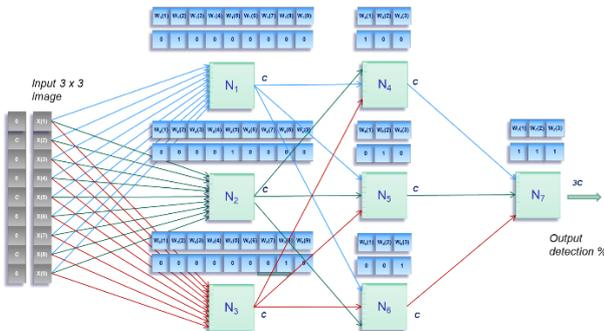
Figure 11. Architecture: 2 layers of 3 neurons
