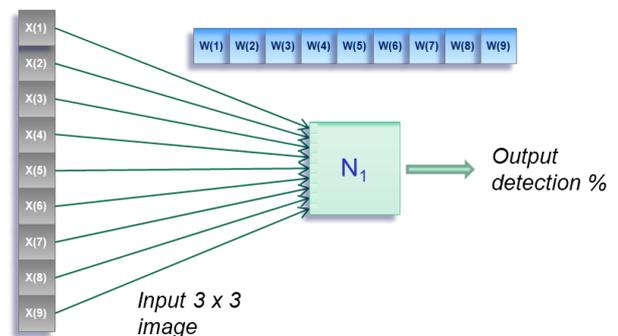
Figure 9. Simplest architecture: 1 layer of 1 neuron
