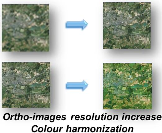
Figure 22. Example of ortho-image improvement
