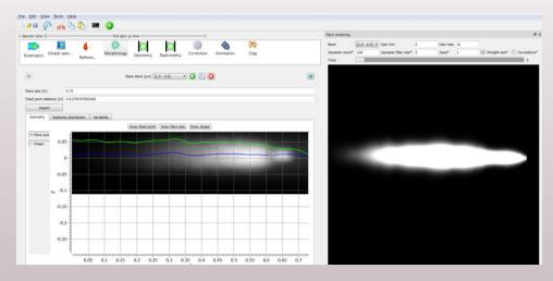
As the physical structure and the dynamics of flare core are too complex to be computed by physical laws, the SE-FLARE interface proposes to create a simulated core starting from measurement data. Thermography in several wavebands can be loaded and displayed in this interface. Then the enduser can re-create similar shapes by an interactive process.
