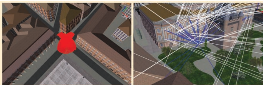
FIGURE 4 Left: obscuration representation. The receiver is located at the center of the red virtual sphere. Right: example of GPS reception close to the City Hall of Toulouse, France. In white, incoming rays from the satellites, in blue, diffracted rays, in red reflected rays (simulation)
