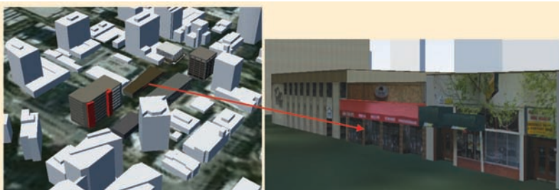
FIGURE 6 The synthetic environment models a narrow street. White buildings are defined in low resolution. Buildings close to the receiver are detailed in order to model the influence of small structures on the reception.
