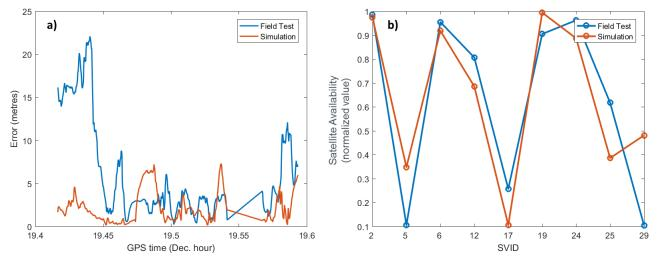
Figure 12. (a) Positioning error for field-test (blue) and simulation (red); (b) Satellite availability for field data (blue) and simulation (red) after scene improvement.
