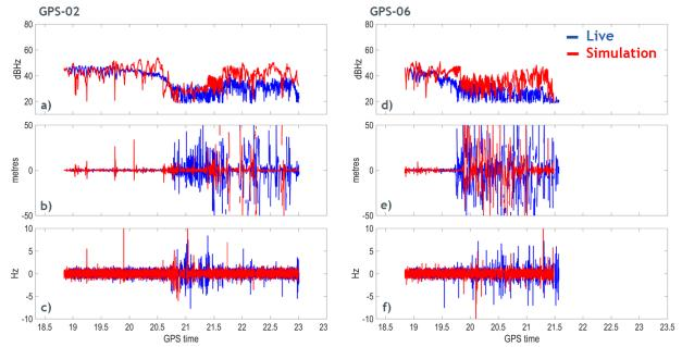
Figure 6. Carrier-to-Noise ratio (top), pseudorange residual (middle), and doppler residual (bottom) for PRN 02 (left column) and PRN 06 (right column).
