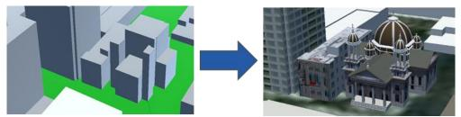
Figure 5. Improvement (right) in a San Jose building since its complexity in the architecture was believed to generate more reflections than the ones obtained with a more simplistic box model (left).
