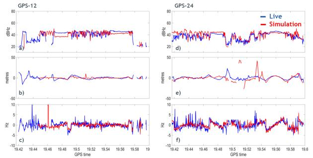
Figure 11. Carrier-to-Noise ratio (top), pseudorange residual (middle), and doppler residual (bottom) for PRN 12 (left column) and PRN 24 (right column).
