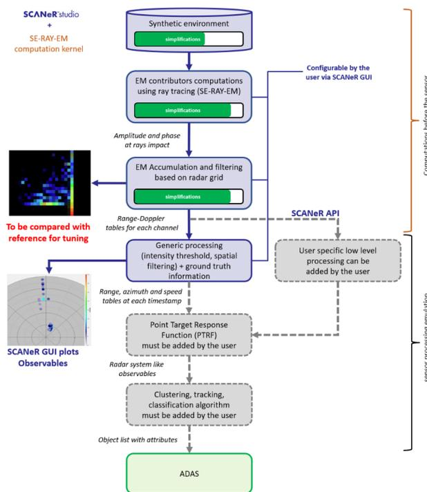
Figure 6: Optimized level - processing steps
