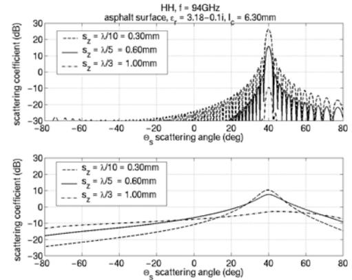
Fig. 4 : Coherent and incoherent bistatic scattering from asphalt at 94GHz
