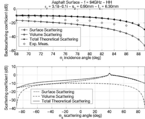
Fig 6 : HH asphalt total scattering coefficients
