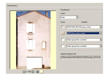
For each layer, a material modulation is computed, and a *EM* pre visualisation enable to check the *EM* consistency of the physical material allocation, as shown hereafter:
