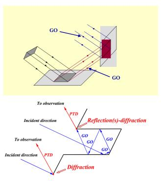
Thus, the scattering of intercepted surfaces throughout the multiple bounces, edge diffraction, reflection(s)-diffraction and/or diffraction-reflection(s) coupling could be considered.
