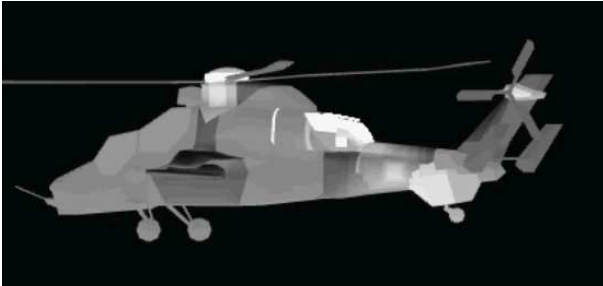
Figure 26. Predicted IR signature of helicopter
