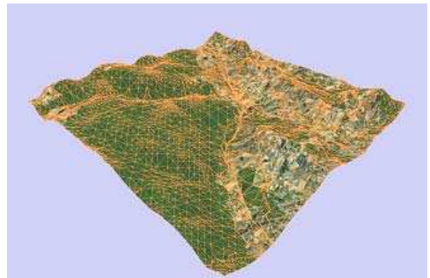
Figure 8. Example of terrain skin mesh
