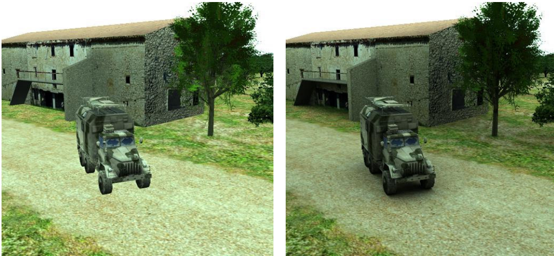
Figure 4: Visible rendering of a scene with a cloud covered atmospheric file using the current version of SE-RAY-IR (left) and the future version with advanced rendering (right).
