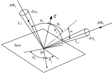
The BRDF (Bi-directional Reflectance Distribution Function) is the only serious data that can be used in physical simulation. It is defined as :
