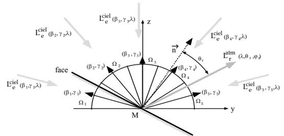
If N is the degree of tessellation, the directional reflected energy for each polygon i, due to sky radiance is computed as :
