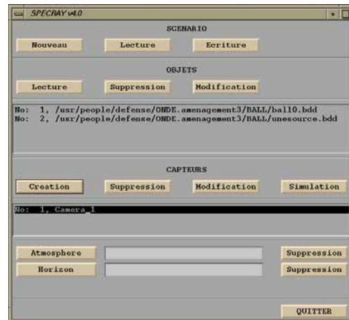
The object panel enables to define the position and Euler angles of each object when static, or the associated path when dynamic (moving objects). The object can be assigned to automatically follow the terrain altimetry using the « Roulement » button. This panel also allows to define light sources.
