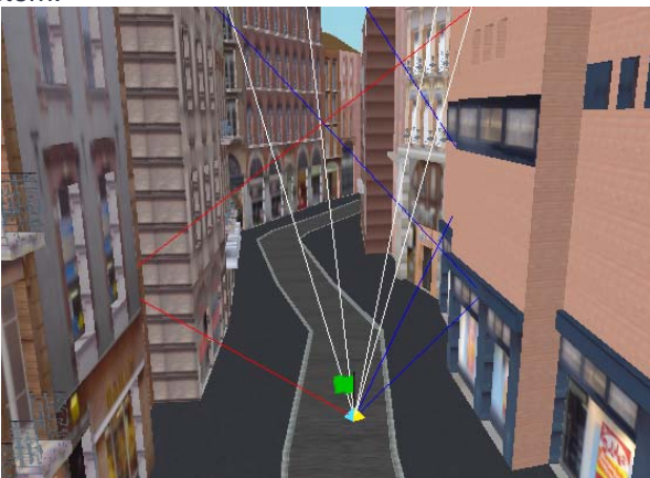
SE-NAV simulation in Toulouse downtown. White rays model the direct paths of the GPS satellites seen by the receiver. Blue and red rays are multipaths.
